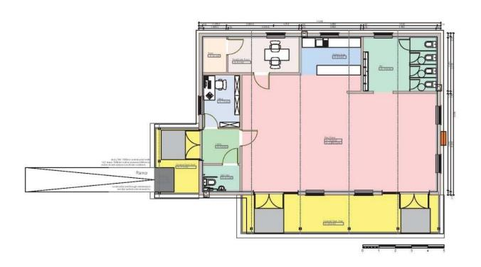
Site conditions are indicative only: indicative plan layout. Furniture shown for purposes of illustration. Internal structural height: 2500mm Total Floor Area (including linings and partitions): 137.3sqm Vertical timber cladding. Aluminium window frames.
